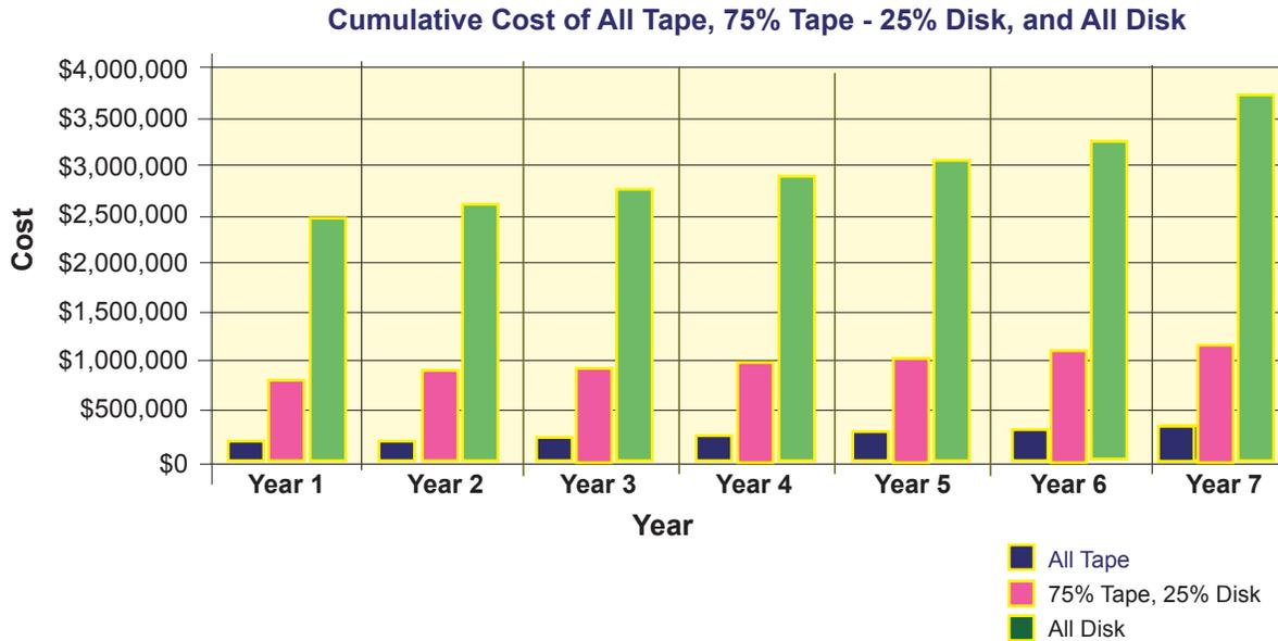
The total cost of the hybrid disk/tape solution, which stores 25% of the backup data on disk and the remaining 75% on tape, is significantly less than the all-disk option, and it has room to grow. The tape library can accommodate an additional 218 cartridges as users' capacity requirements increase.
